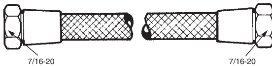
Figure 2-19. Stainless Steel Actuation Hose. 000433
