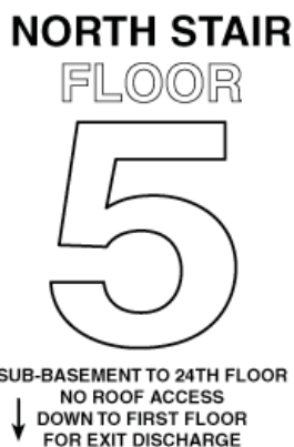
Figure 3.24- Example of a stairway marking sign
