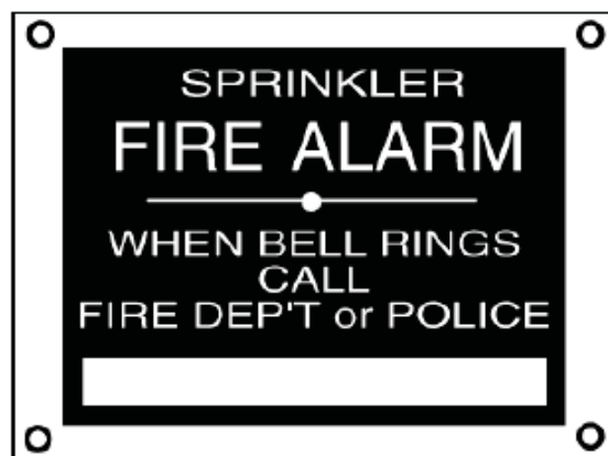
Figure 9.18: Alarm Identification Sign
